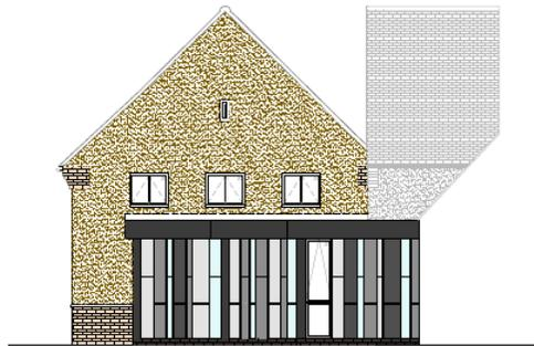
Proposed rear elevation of classroom also showing side elevation of link corridor
